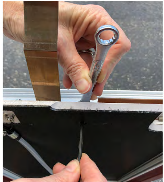
2. Use 1/8" Allen wrench and 3/8" open end wrench to loosen the brown screw shown above.
