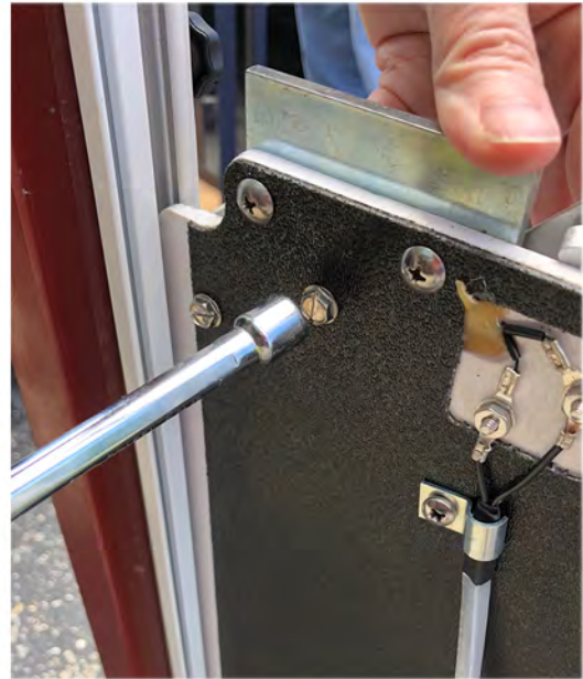
4. Use 5/16 nut driver to unscrew the hex head screws on the lock bracket.
