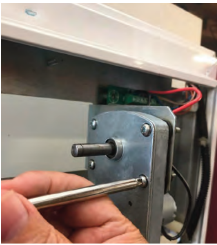
Step 9 - Unscrew phillips head screws holding motor gear box to chassis arm.
