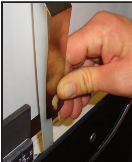
Step 13 - Rehook spring strap to screw post on closing panel.
