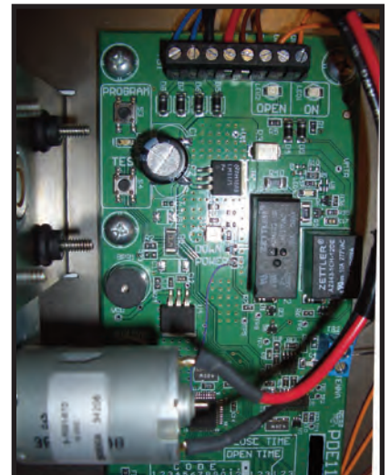
Step 14- Reattach red and black motor wires to circuit board.
