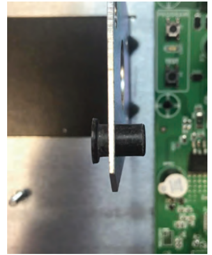
Step 10 - Put on new rubber jacketed nuts as shown above, pushing them through the holes in motor chassis plate arm.
